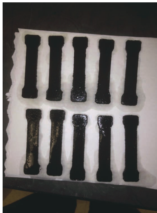
Figure 8. Dogbones after 24 h soaking. [Color figure can be viewed in the online issue, which is available at wileyonlinelibrary.com .]
